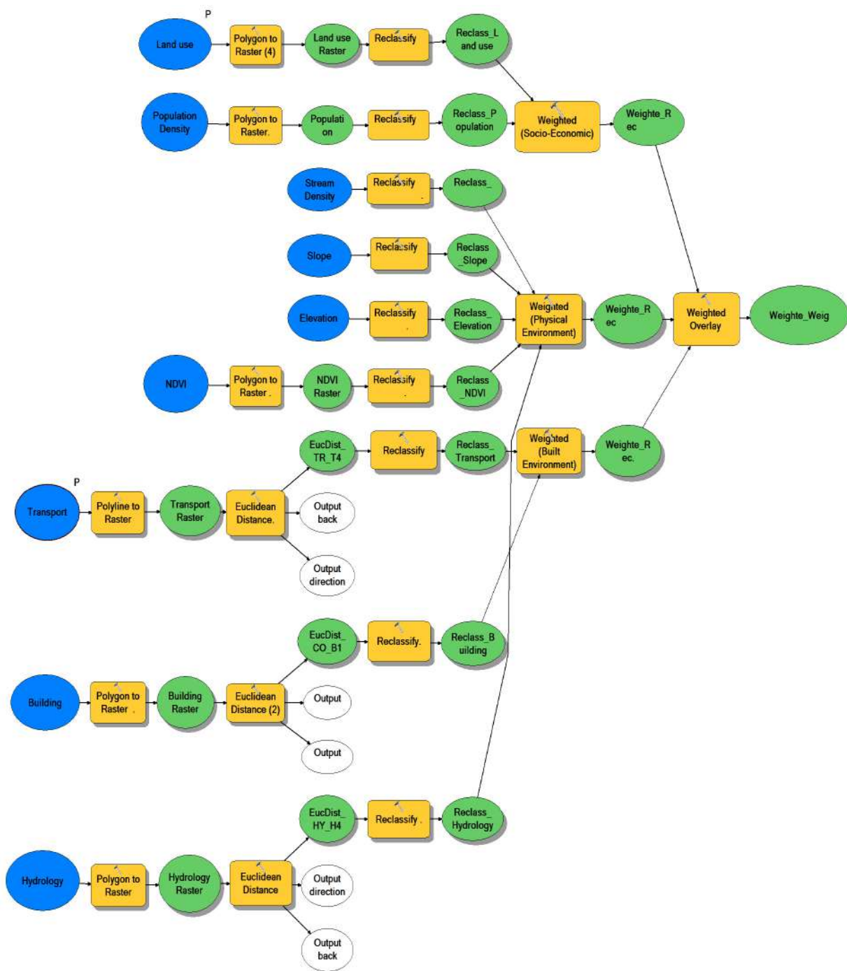
Figure 4. ArcGIS model for creating flood vulnerability map of the Neluha DSD using Model Builder.
